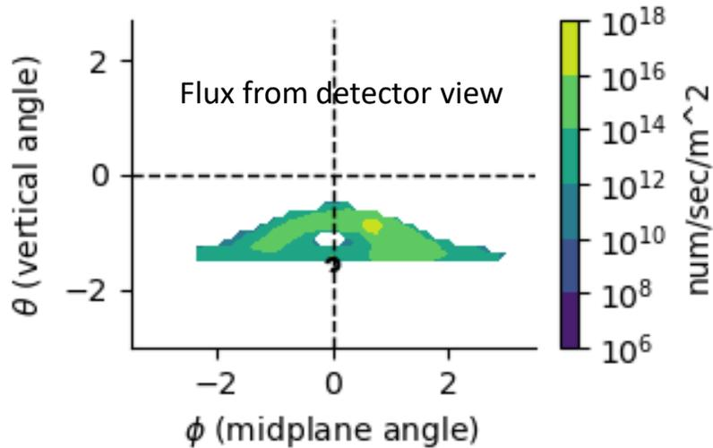
Flux visible to detector location (overhead)
