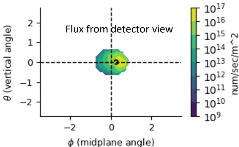
Flux visible to detector location (overhead)
